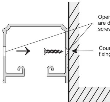
Side fastening of URSUS track - max. weight of 50 kg per door
